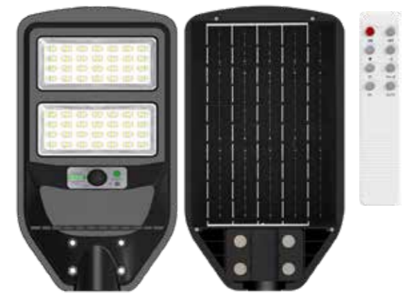
YLD-036912 Panel solar policristalino Size: 211*299mm, glass 2.0mm, power 8W(-0.5W)/5V
